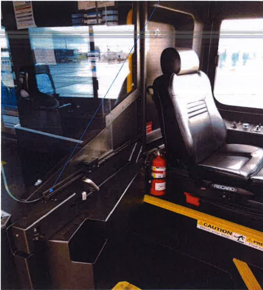
FIXED OPERATOR BARRIERS NEWLEY INSTALLED
