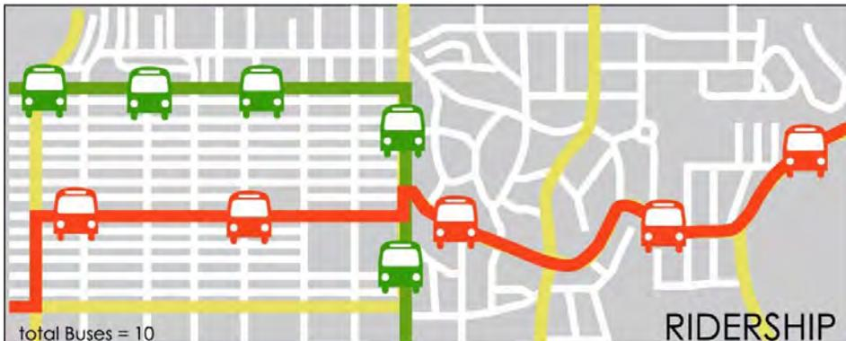
Figure 2: Schematic of coverage network model (fleet of 10 buses)
